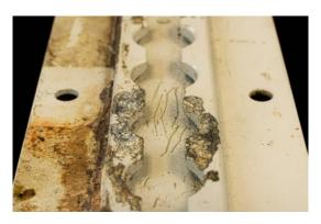
Corrosion is loosely defined as the gradual deterioration of a material's surface through chemical reactions. Though not exclusively reserved for metals, the term is most often applied when talking about metallic components. The corrosive process is affected by a myriad of factors, including environment, product design, storage, cleaning, and mating surfaces.
